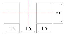
Unit: mm Tolerance: ± 0.10mm
