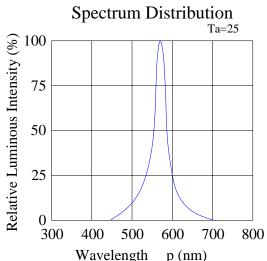
Wavelength p (nm) Luminous Intensity &
