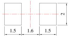
Unit: mm Tolerance: ± 0.10mm
