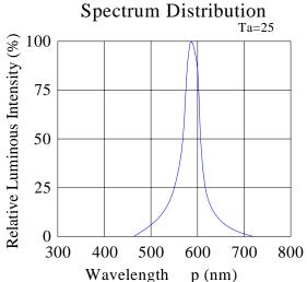
Wavelength p (nm) Luminous Intensity &
