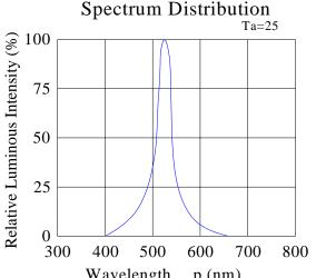
Wavelength p (nm) Luminous Intensity &
