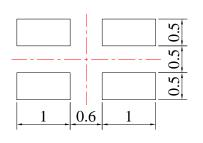
Unit: mm Tolerance: ± 0.10mm
