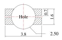
Unit: mm Tolerance: ± 0.10mm
