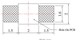
Unit: mm Tolerance: ± 0.10mm
