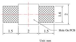
Unit: mm Tolerance: ± 0.10mm
